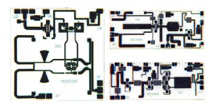
MEC has successfully completed a number of shared multi-project GaAs wafer with the UMS foundry.
